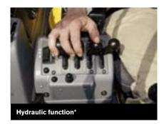
The hydraulic system in the L90E is prepared for installation of a third hydraulic function. The separate third hydraulic function with its control lever and additional lines can easily be installed to further increase the loader's flexibility.
