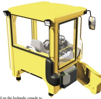
wheel and on the hydraulic console to the right. With CDC (Comfort Drive Control)\*, the operator can operate steering, forward-reverse and kickdown function with controls in the left armrest. At any time, the operator can switch between steering with the steering wheel and CDC, which helps to minimize tiring and repetitive movements. This gives the operator the possibility to vary operating mode and reduce fatigue and static muscle strain.
